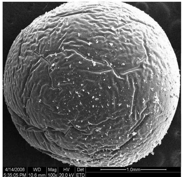
Fig. 1 – SEM photograph of the surface of the alginate gel beads (85 \times )
