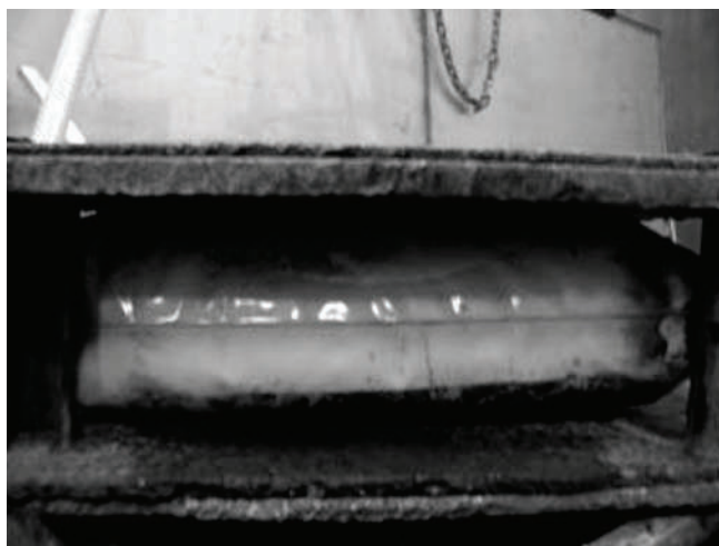
Figure 4 Schematic presentation of the experimental set-up for double hull construction, outer hull 14-19 mm thick, inner hull 12-14 mm thick
