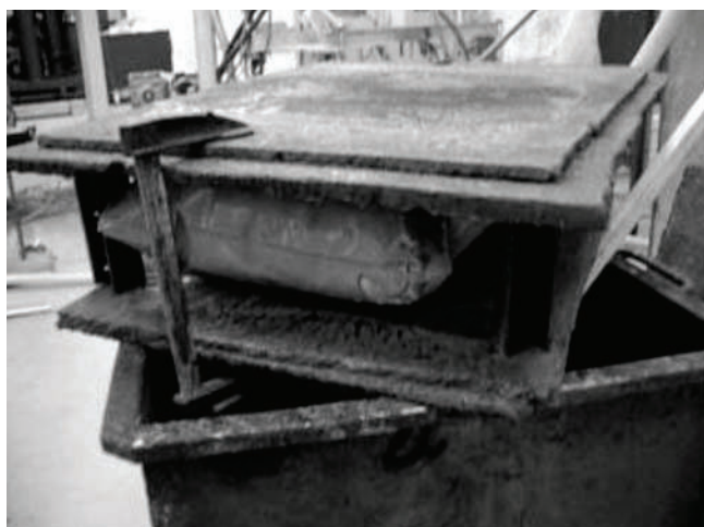
Figure 5 Double hull construction, the air bag is placed between two iron plates so that the whole set-up can be immersed in water
