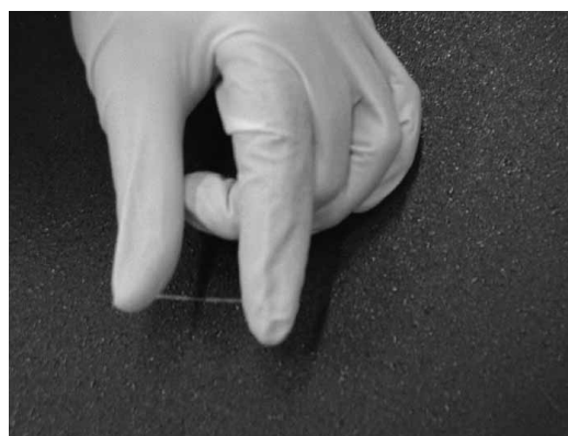
Fig. 2. Viscosity test – it is low (the string is shorter than 3 cm).
