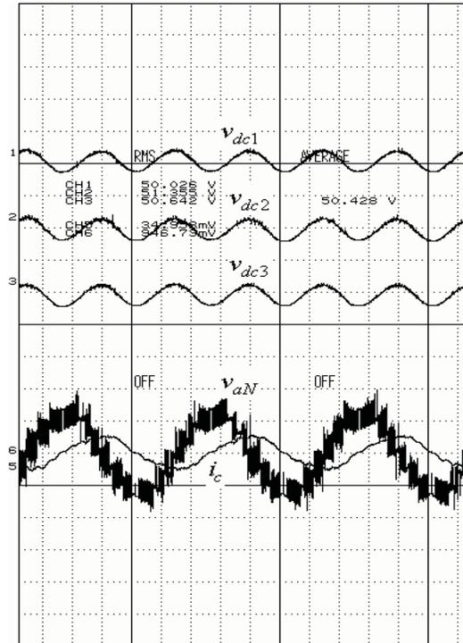
Fig. 14. Experimental results of the multilevel DSTATCOM for the lagging reactive current
