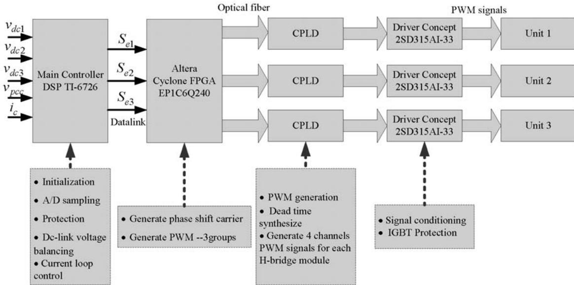
Fig. 2. Proposed controller architecture for the multilevel DSTATCOM
