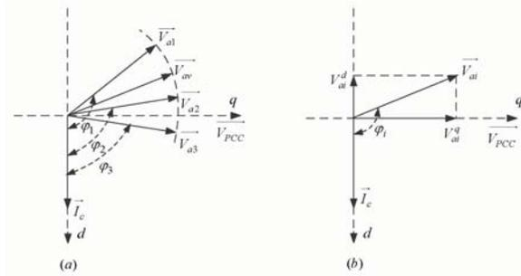
Fig. 7. Phasor representation of the individual H-bridge voltage with respect to its injection current
