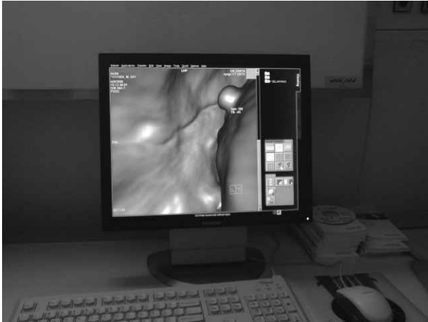
Fig 1. Dual Xeon Fujitsu-Siemens workstation equipped with HRCT data postprocessing software Syngo 3D 2006G.
