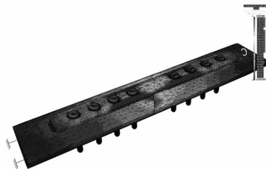
Fig. 4. Numerical model of contact surface in modified osteosynthesis.
