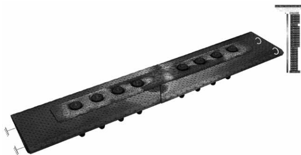
Fig. 3. Numerical model of contact surface in standard osteosynthesis.
