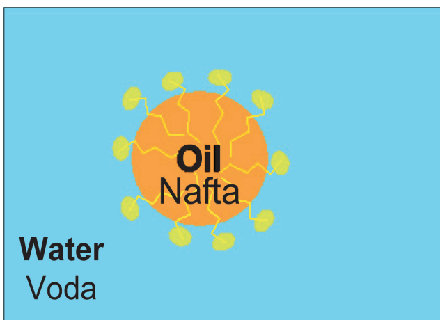
Fig. 1. The mechanism of surface-active agent to create oil in water emulsion
