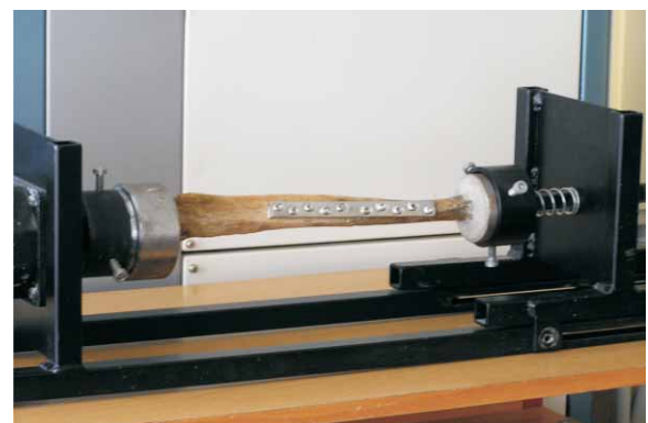
Figure 1b. Picture of the device for static and dynamic research on long bone models.
