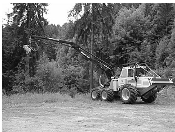
Fig. 4 LKT 120 T-H, special forestry machines, intentionally designed for tree cutting, branching and bucking to the desired length
