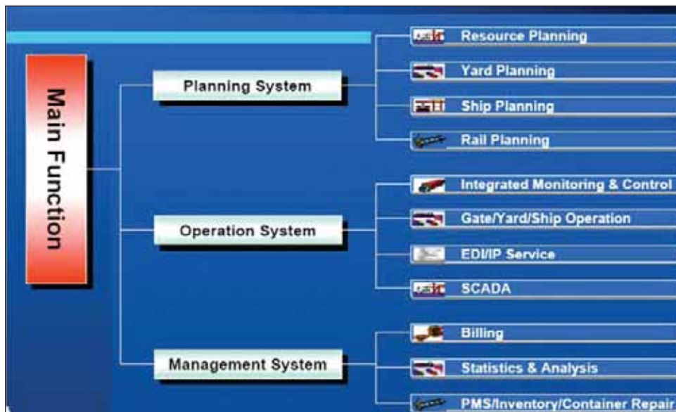
Fig (7) – The modules of modern terminal operating system Slika 7. Moduli modernoga radnog sustava terminala
