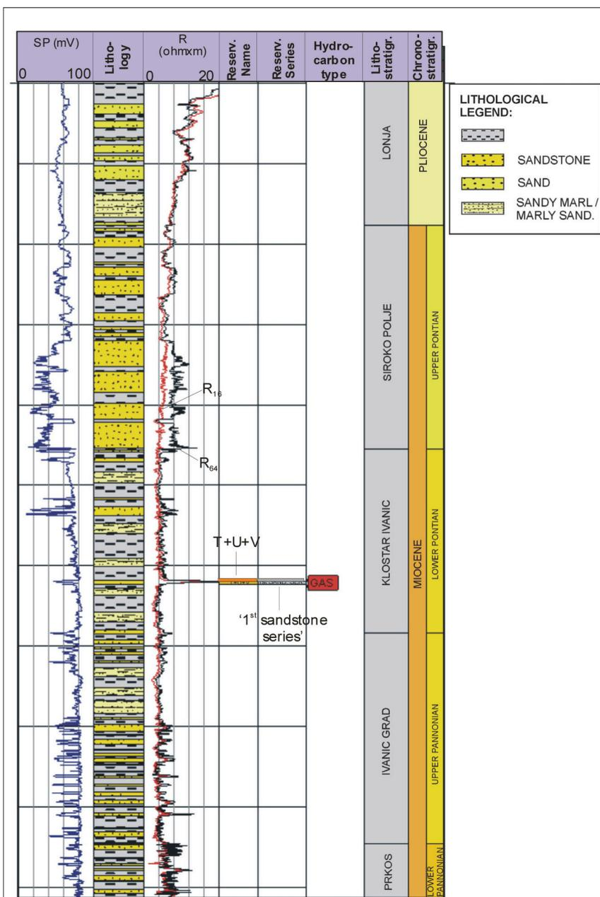
**Fig. 1. Composite geological column (including stratigraphy, e-logs and lithology) of the well with minimum average porosity in the analysed sandstone reservoir 'T' (location belongs to sandy marl lithofacies)**
