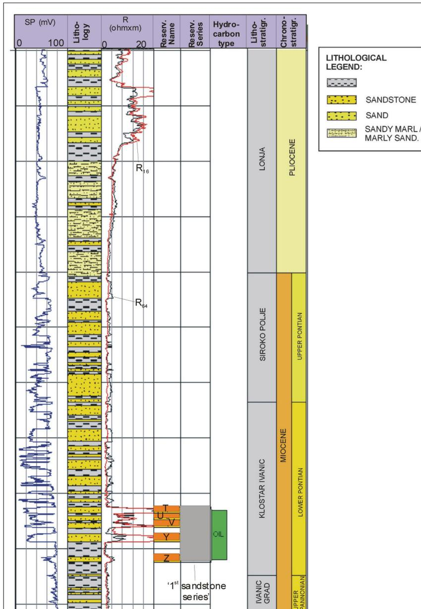
**Fig. 2. Composite geological column (including stratigraphy, e-logs and lithology) of the well with maximum average porosity in the analysed sandstone reservoir 'T' (location belongs to medium grained sandstones lithofacies)**
