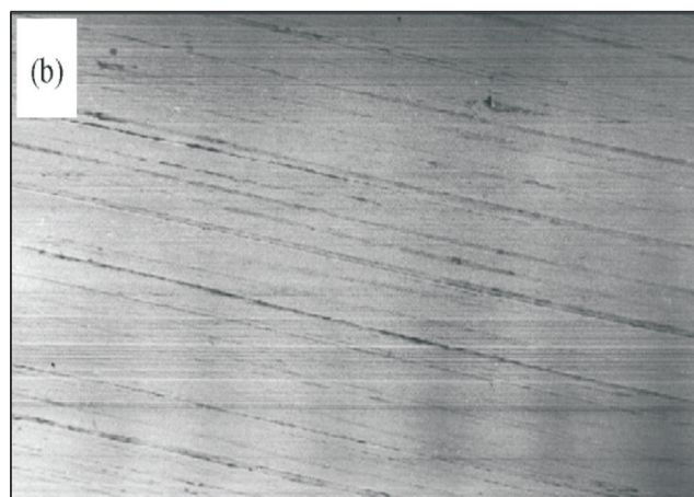
Plate 8. Clean coupon surface at (350 °F) (177 °C), pH 5.5, 50 mg/l sulphide, 100 mg/l ferrous gluconate.. Focus: ×100
