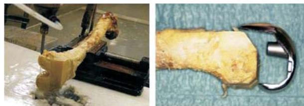
Figure 4 Division of a bone by the water jet [6] Slika 4. Rezanje kosti vodenim mlazom [6]
