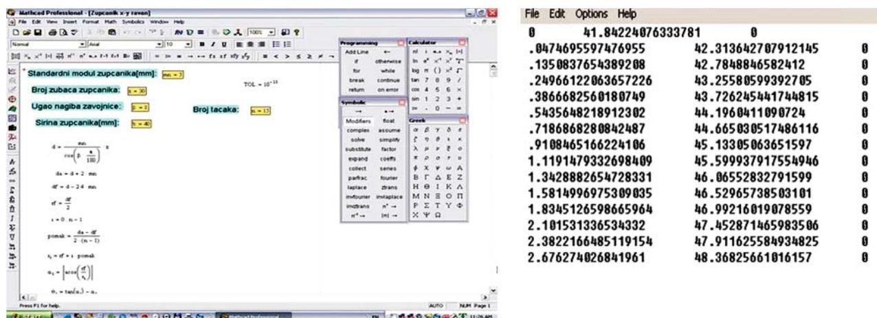
Figure 1 The calculation in MathCad and the results obtained for the evolute calculation in 15 points
