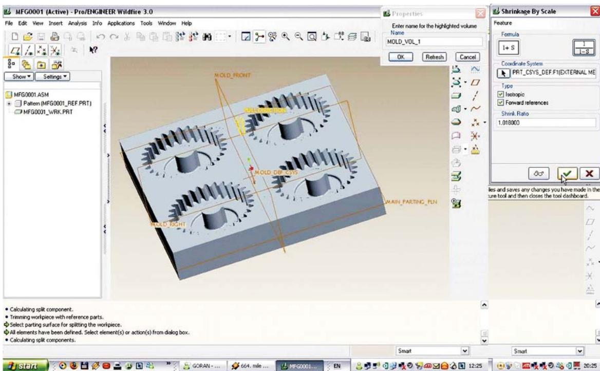
Figure 6 The adopted "shrinkage" percentage of plastics based on which the final casting panel model was created
