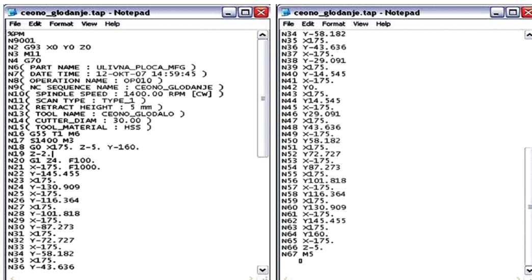
Figure 7 The presented part of the G-code of the direct steering file
