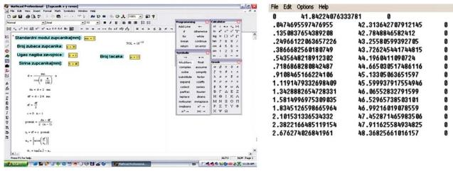
Figure 1 The calculation in MathCad and the results obtained for the evolute calculation in 15 points Slika 1. Proračun u MathCadu i rezultati za proračun evolvente u 15 točaka
