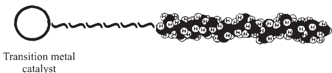
FIGURE 14 – Simplified scheme of the beginning of polypropylene crystallization during coordinative polymerization reaction of propylene 18
