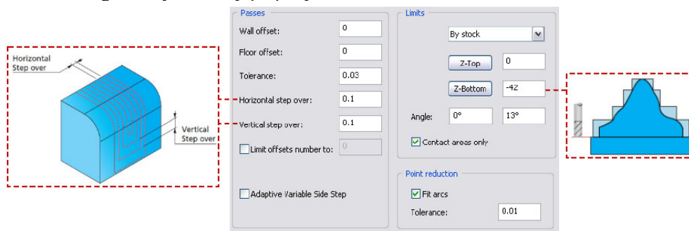
Figure 10. Parameters on the “Passes” technological card for the “Constant step over” sequence
