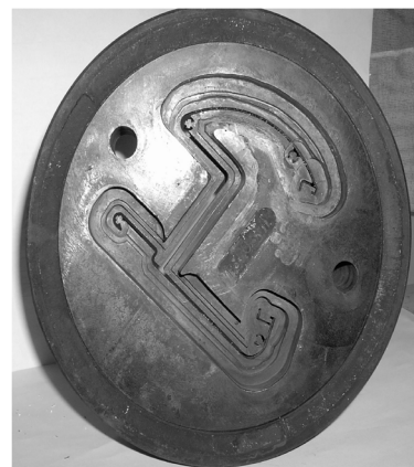
Figure 1. Model of finished part and appropriate tool die Slika 1. Model gotovog dijela i odgovarajuća alatna matrica
