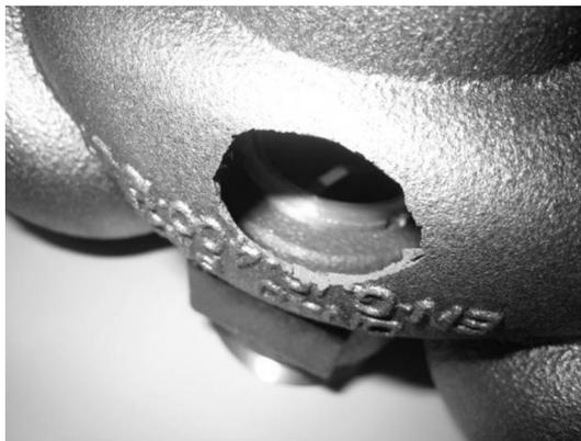
**Figure 14.** Thin upper wall caused by vertical core movement
