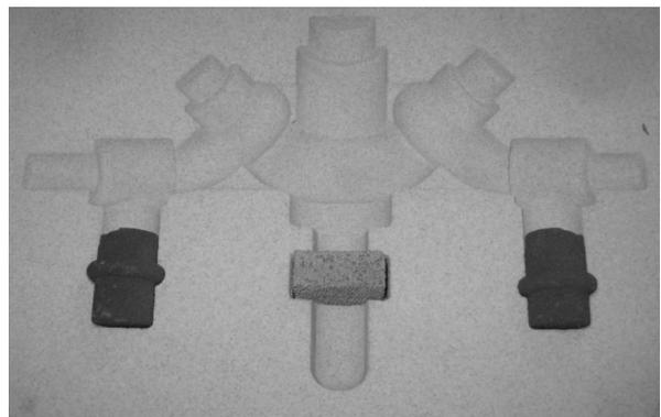
**Figure 9.** Inserting mould cores and filter.
