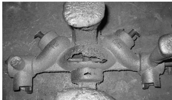
**Figure 12.** Hole in the casting, caused by lifting of the broken core
