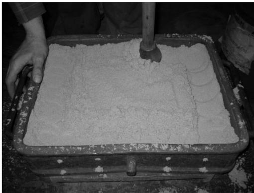
**Figure 5.** The sand is then set and pressed. Used sand is Termit, as binder glass water (3 to 5 %) was used
