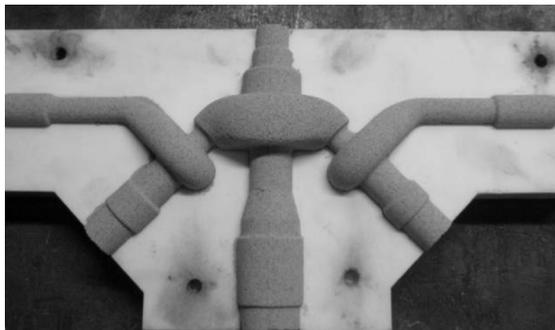
**Figure 17.** Polyamide mould for core manufacturing. A wire was added prior to CO<sub>2</sub> curing in order to reinforce the core
