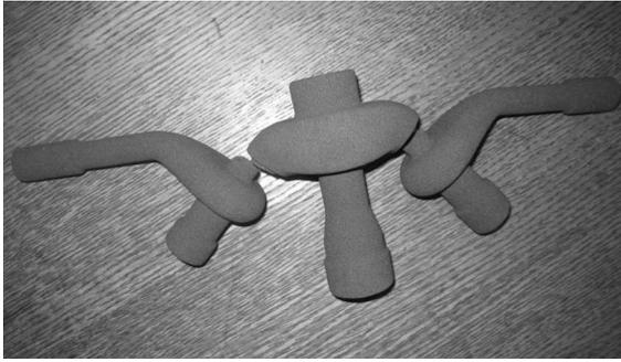
**Figure 13.** Core breaking on part with smallest core thickness
