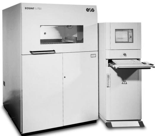
**Figure 2.** The EOSINT S 750 is double laser-sintering system for the processing of Croning moulding material. Using the DirectCast method, the system builds cores and moulds for sand casting
