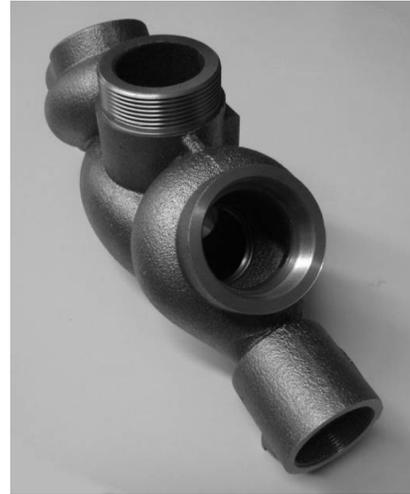
**Figure 11.** Casting after final machining
