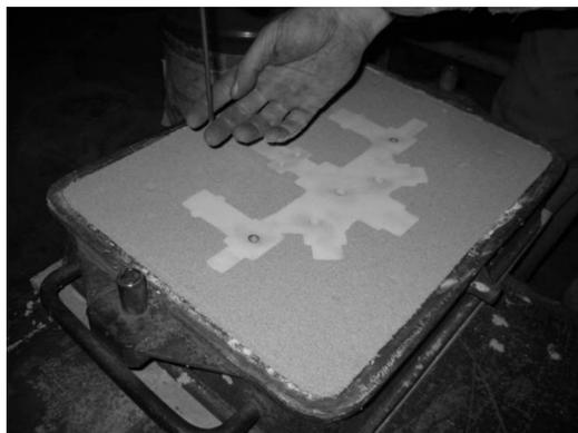
**Figure 6.** Curing of the sand form with CO2 gas
