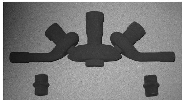
**Figure 8.** Sand cores made with Generis Sand Process on S 15 machine.
