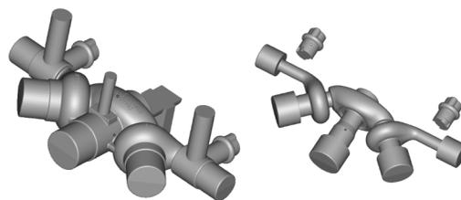
**Figure 1.** Left: CAD model of the valve with added attachments and feeders used for SLS (Selective Laser Sintering) manufacturing from polyamide. Right: CAD model of a valve's core used for GSP (Generis Sand Process) manufacturing
