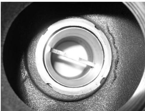
**Figure 15.** Problems of CNC machining due to valve opening not being coaxial
