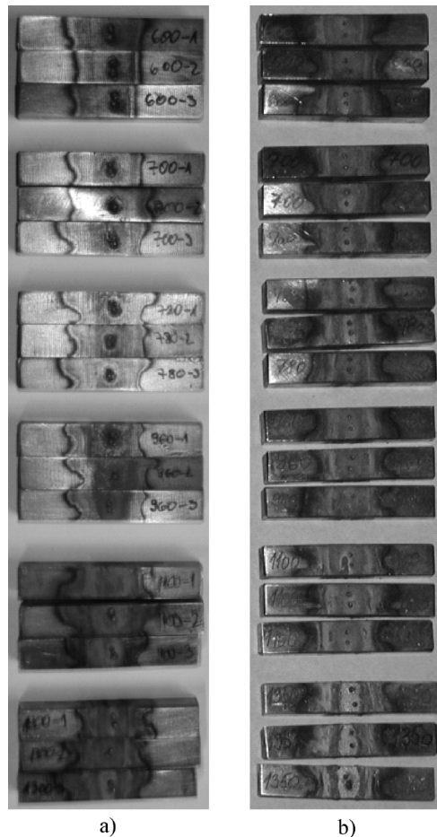
Figure 8. Single thermal cycled (a) and double cycled (b) specimens at different peak temperatures in the HAZ
