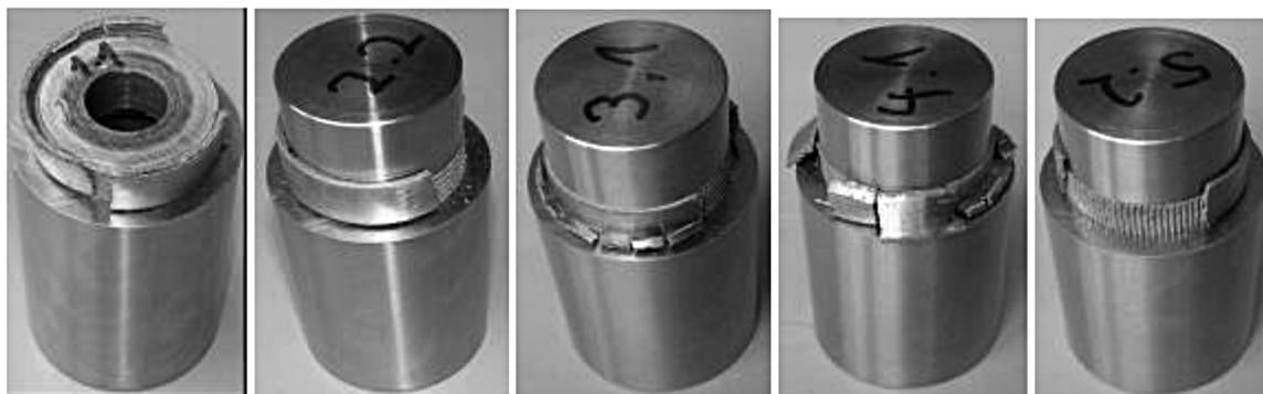
Figure 7. Typical appearance of the specimens after shear testing
