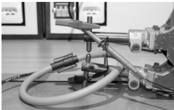
Figure 7. Working place: a) connection to laboratory desk; b) connection of Rogowski coil and oscilloscope clamps for voltage measurement
