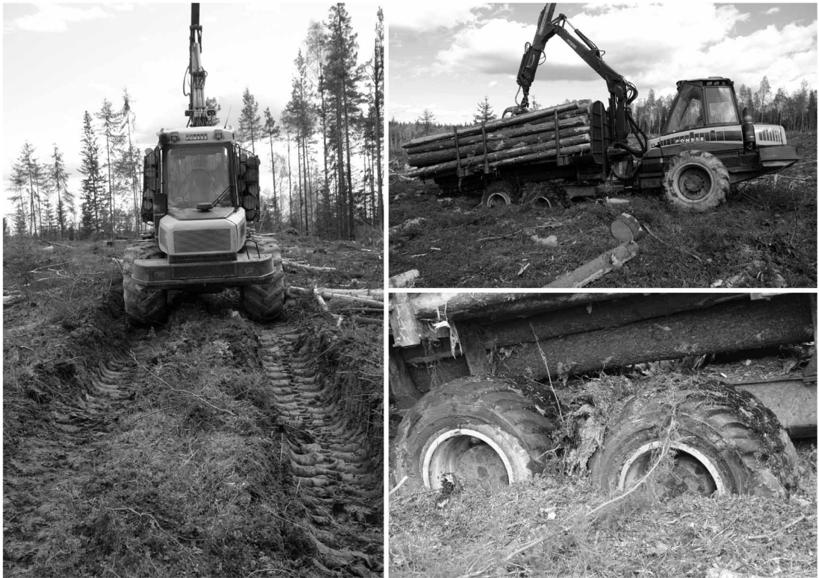
Fig. 1 Typical rut on silt loam soil caused by forwarder passes
