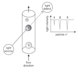
**Figure 2:** Schematic illustration of the particle counter. The water sample passes through a tube illuminated by a laser beam. Every particle (1, 2, 3) creates a "shadow" observed at a light detector, which makes it possible to determine the number and size of the particles.
