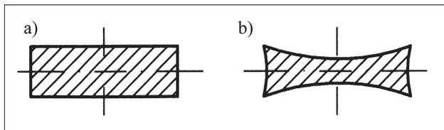
Figure 2 Cross-sectional area in the neck at fracture: a) before fracture, b) after fracture
