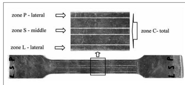
Figure 3 Tensile specimen with marked control lines
