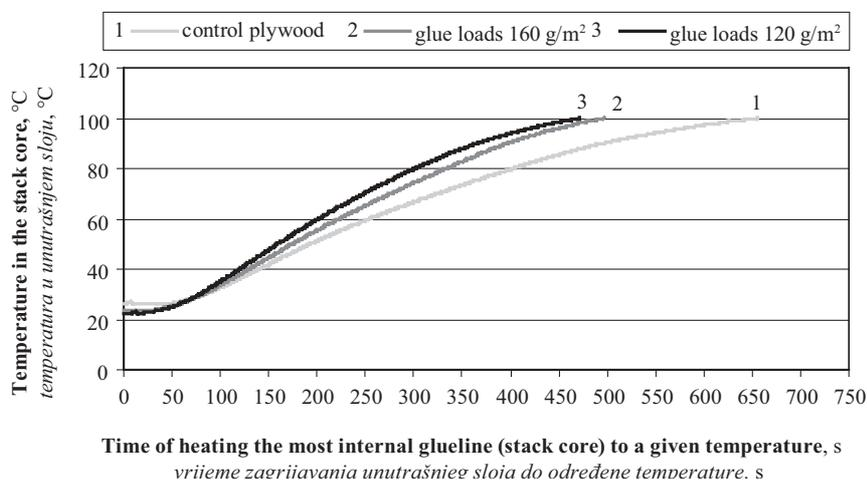
**Figure 1** Overheating times determined for 20 mm plywood made of densified pine veneers
