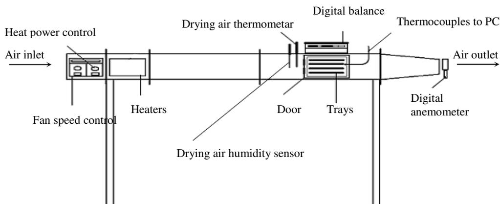
Fig. 1. Laboratory dryer used for convective drying
