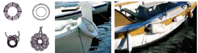
Figure 22 **Rubbing strips: rolled up ropes, automobile tire and strong plastic material**
