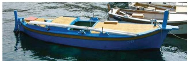
The flooring made of quality wood is provided, by which all the bottom space, above floors, is covered. The bail with a handle (volume 1-1.5 lit.) is carved from a very thick piece of wood for bailing out sea water from the boat's bottom. When the boat is finished, the launching ceremony follows and the boat is named and launched gliding down the slide bearing (building berth) or it is lifted and lowered in the sea by a boat crane or an automobile crane.
