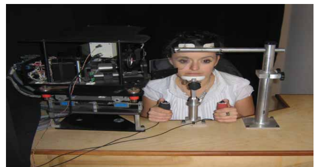
Fig. 11. »Dual Purkinje Eye tracker« operating according to the principle of reflection of lights positioned in front of the lens and behind the lens.
