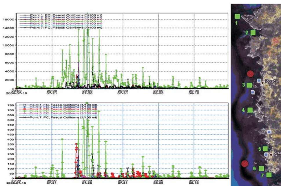
Figure 12 Dynamics of concentration of faecal coliforms at points 300 m from shore (top left panel: present status of development, bottom left panel: planned level of development with use of membrane treatment technology, right panel: red - temperature and salinity measurement points; green - points 300 m from shore with highest concentration of faecal coliforms)
