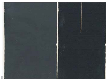
Figure 3 Comparison of sample 2 (zinc phosphate epoxy base coat/polyurethane water cover coat) after 6 months in laboratory (1st plate) and 1008 h testing in salt chamber (2nd plate)
