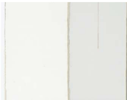
Figure 5 Comparison of sample 4 (zinc phosphate epoxy dispersion/ water polyurethane cover coat) after 6 months in laboratory (1st plate) and 1008 h testing in salt chamber (2nd plate)
