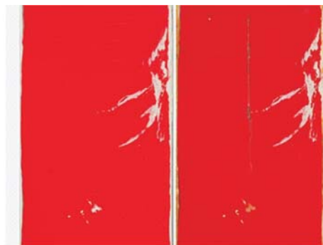
Figure 2 Comparison of sample 1 (zinc phosphate epoxy base coat/polyurethane cover coat) after 6 months in laboratory (1st plate) and 1008 h testing in salt chamber (2nd plate)
