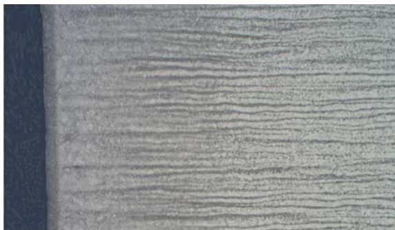
Figure 5 The HAZ transition after the oxygen cutting – magnification 100× Slika 5. Prijelaz ZUT-a nakon plinskog rezanja – povećanje 100×
