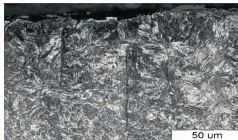
Figure 9 The HAZ transition after the plasma cutting – magnification 500× Slika 9. Prijelaz ZUT-a nakon rezanja plazmom – povećanje 500×
