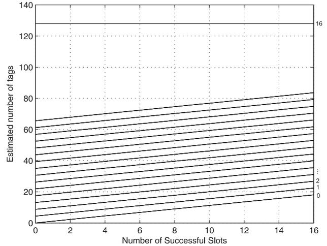
Fig. 7. Linear model behavior of the frame ( $L = 16$ ) obtained from combinatorial model. Lines represent collisions, 0 – 15, down-up. Last line, for all collision scenario is in this case  $n = 2^{Q_{current\ frame} + 3} = 2^7 = 128$
