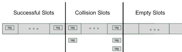
Fig. 4. After reader interrogation, we arrange the frame in the successively array of Successful, Collision and Empty Slots
