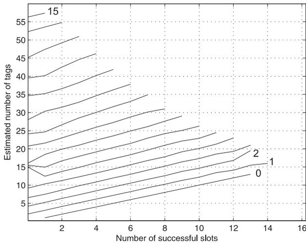
Fig. 6. Linear model behavior of the frame ( $L = 16$ ) obtained experimentally in [21]. Lines represent collisions, 0 – 15, down-up. 16<sup>th</sup> line is a point, because all-collision scenario results with 0 successful slots
