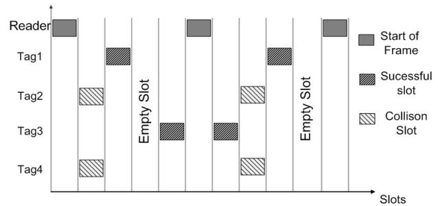
Fig. 1. Example of Framed Slotted ALOHA protocol with length of frame equal to 4, and 4 tags within interrogation area
