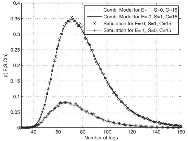
Fig. 5. Results of FSA simulation and Combinatorial model in (14). The maximum of depicted distributions  $p(E, S, C | n)$  is used as estimation of number of tags within interrogation area.
