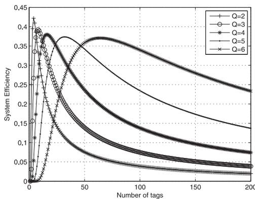
Fig. 2. FSA efficiency for different frame lengths
