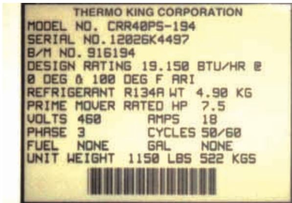
Slika 4. Tablica s podacima o rashladnoj jedinici Figure 4. Table with the data on the refrigerating plant
