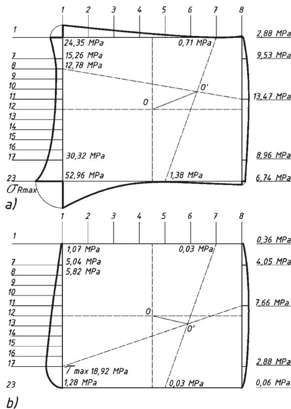
**Figure 7** Stress distribution in the rectangular glue bond: a) reduced stresses according to Von Mises, b) shear stresses  $\tau_{xz}$ ,  $\tau_{xy}$
