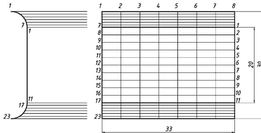
**Figure 5** Measurements of glue bond and designations of stress measurement points
