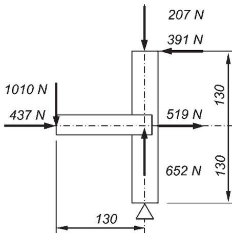
**Figure 3** Loading diagram of the back leg joint with the connecting bar
