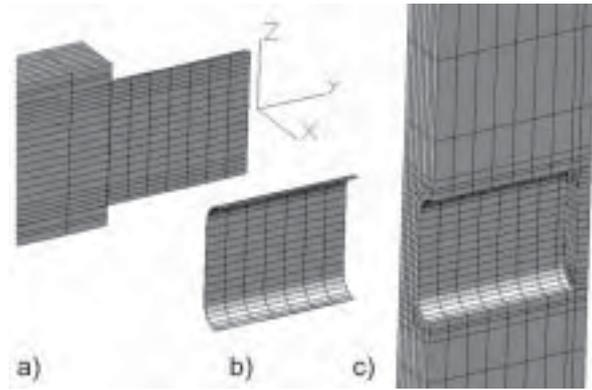
**Figure 4** Numeric model of the tenon joint: a) tenon, b) glueline, c) mortise
