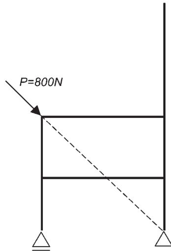
**Figure 2** Static diagram of the chair construction loading
