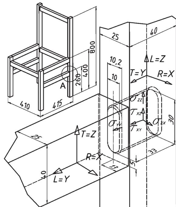
Figure 1 Measurements of the chair and tenon joint
