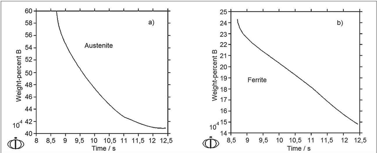
Figure 5 Concentration of B in austenite a) and ferrite b) in the grain boundary area  $\gamma/\alpha$  at  $V_c = 50$  °C/s
