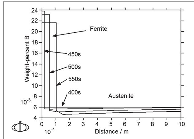
Figure 1 Concentration of boron in the function of distance in  $\gamma/\alpha$  phase area after simulation time 400, 450, 500 and 550 s at cooling rate  $V_c = 1$  °C/s
