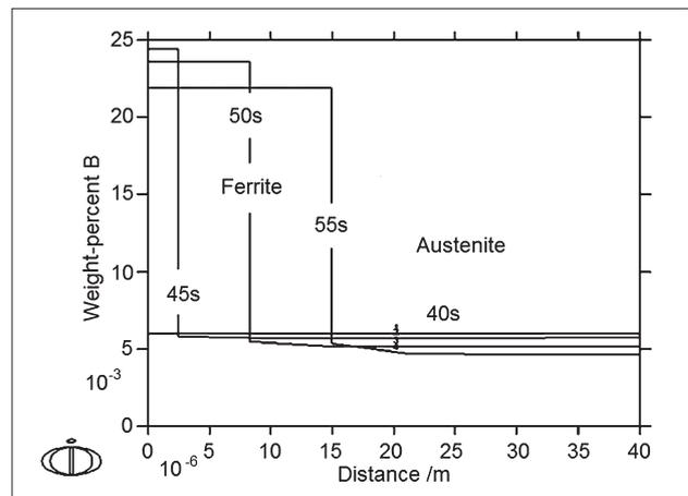
Figure 2 Concentration of boron in the function of distance in  $\gamma/\alpha$  phase area after simulation time 40, 45, 50 and 55 s at cooling rate  $V_c = 10$  °C/s
