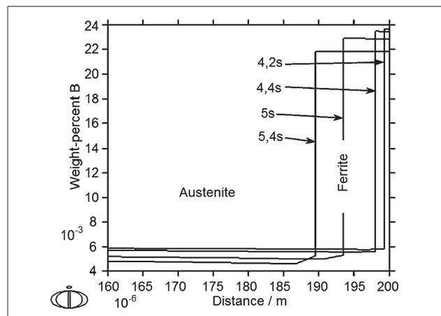
Figure 3 Concentration of boron in the function of distance in  $\gamma/\alpha$  phase area after simulation time 4,2-5,4 s at cooling rate  $V_c = 100$  °C/s
