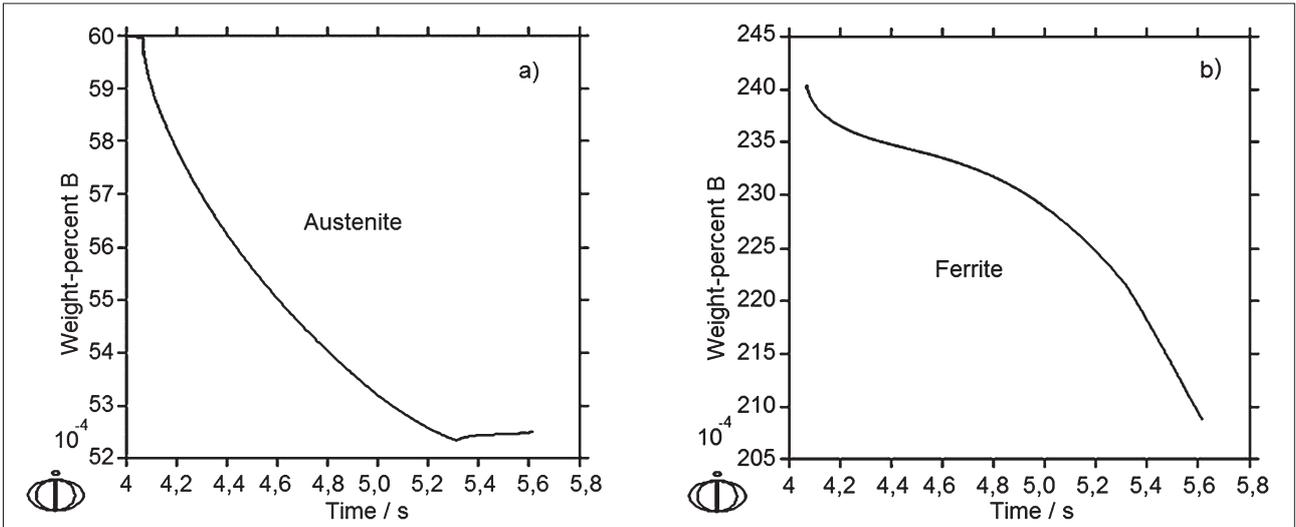
Figure 4 Concentration of B in austenite a) and ferrite b) in the grain boundary area  $\gamma/\alpha$  at  $V_c = 100$  °C/s
