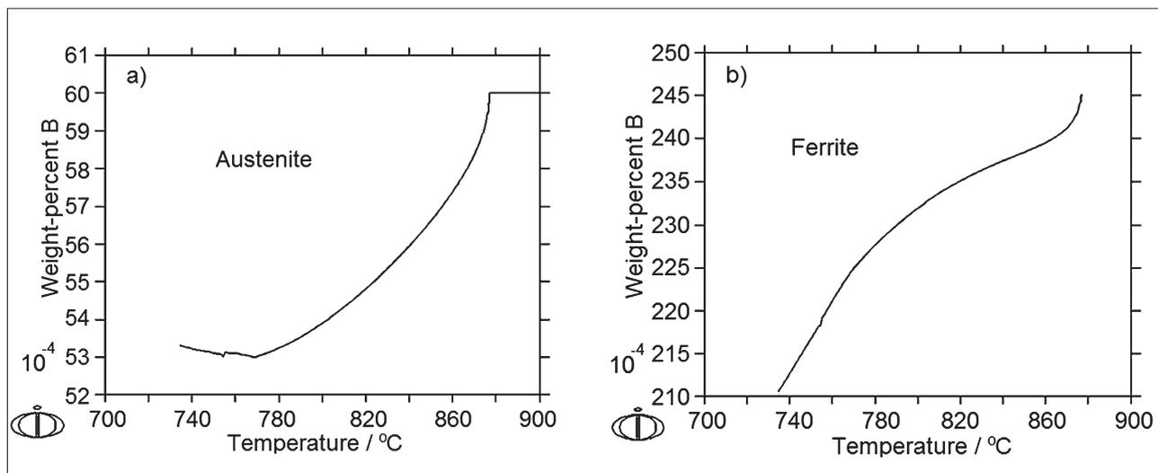
Figure 7 Concentration of B in austenite a) and ferrite b) in the grain boundary area  $\gamma/\alpha$  at  $V_c = 1$  °C/s
