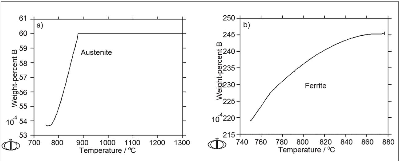
Figure 6 Concentration of B in austenite a) and ferrite b) in the grain boundary area  $\gamma/\alpha$  at  $V_c = 10$  °C/s
