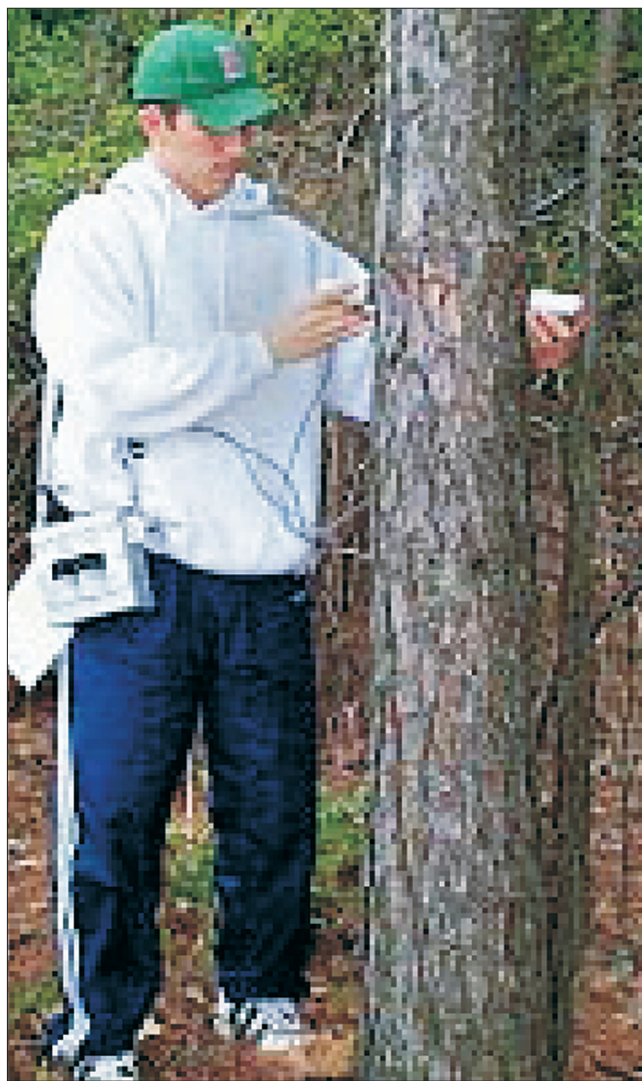
Figure 3 Using ultrasound to detect defects in trees. Slika 3. Otkrivanje grešaka u stablu pomoću ultrazvuka. (Source/Izvor: Leininger et al. 2001)
