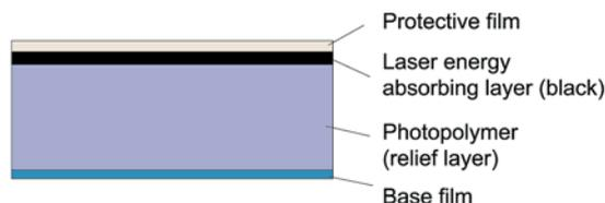
Figure 1 Structure of the CtP flexographic plate
