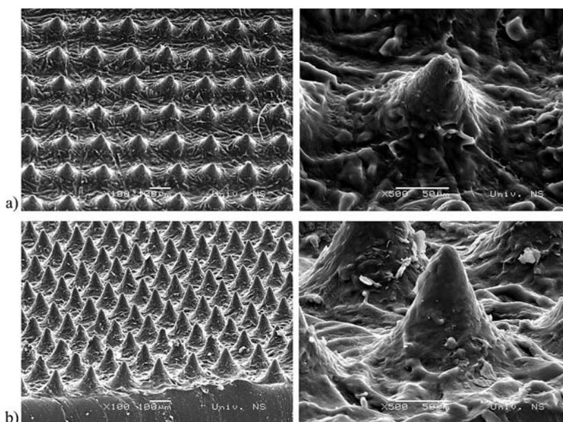
Figure 7 SEM images of 1 % of coverage (a) main exposure 12 minutes; thermal processing carried out with the 8 rotations of the drum and (b) main exposure 12 minutes; thermal processing carried out with the 10 rotations of the drum (magnification 100 and 500×, respectively)
