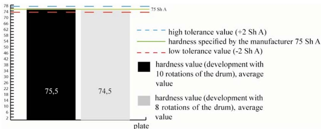
Figure 11 Printing plate hardness, mean value
