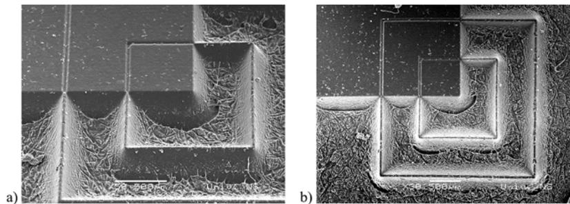
**Figure 9** SEM micrographs of the positive and reverse cross lines of 0,03 and 0,04 mm.
