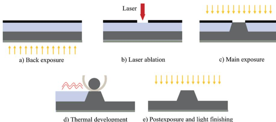
Figure 2 Imaging and thermal development of photopolymer plates
