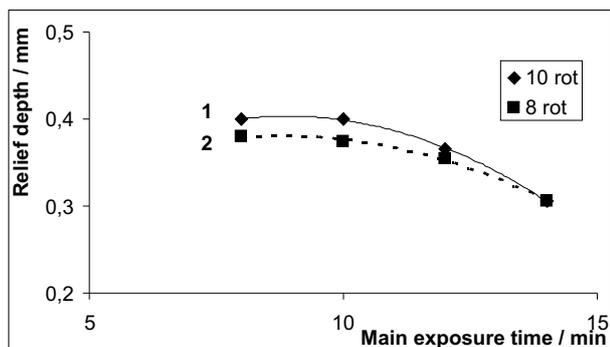
Figure 6 Dependence of relief depth on main exposure for thermal development of 8 and 10 rotations of the drum
