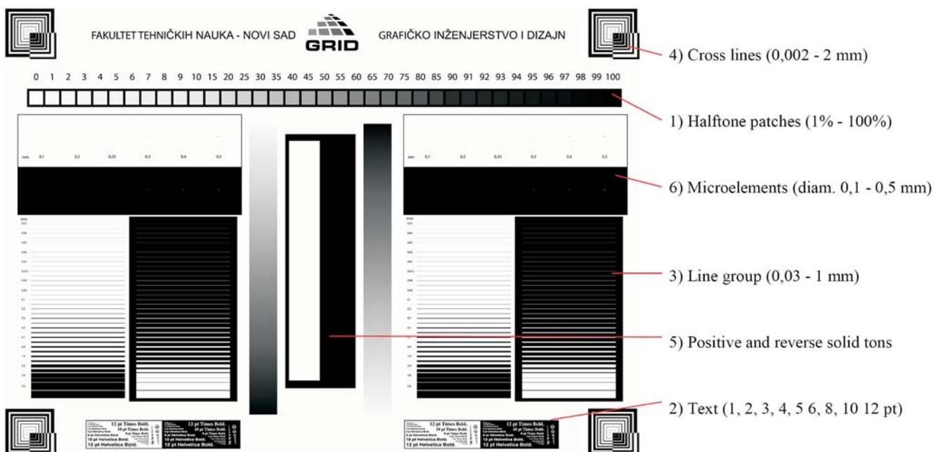
Figure 4 Digital test form
