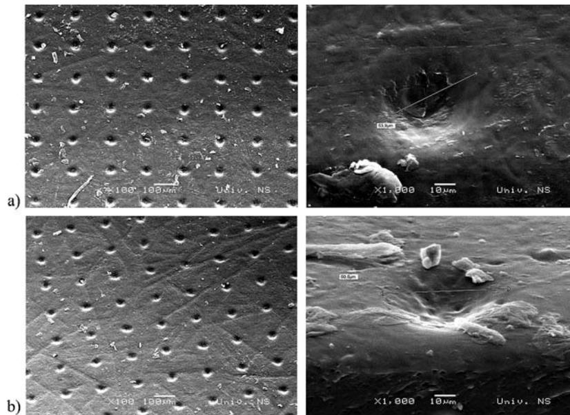
**Figure 8** SEM images of 98 % of coverage (a) main exposure 12 minutes; thermal processing carried out with the 8 rotations of the drum and (b) main exposure 12 minutes; thermal processing carried out with the 10 rotations of the drum (magnification 100 and 500 $\times$ , respectively)
