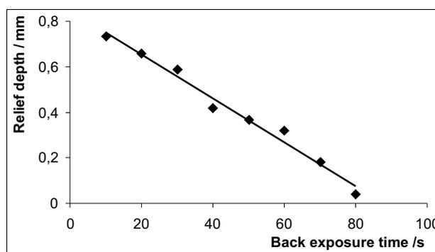
Figure 5 Back exposure test – dependence of relief depth on back exposure duration
