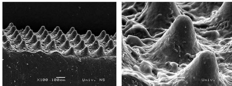
**Figure 10** SEM images of halftone fields (50 % coverage), main exposure 12 min; development 8 rotations of the drum (magnification 100 and 500 $\times$  respectively)
