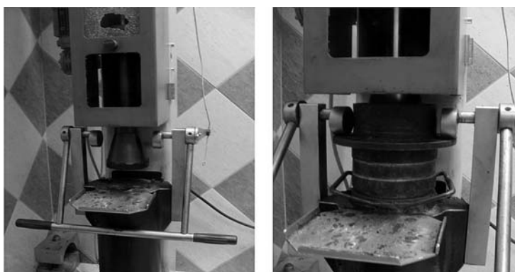
Figure 4 Preparation of samples by impact compactor Slika 4. Priprema uzoraka udarnim zbijračem
