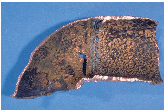
Fig. 6. The "Horseshoe" type erosion-corrosion damage in a copper pipeline.
