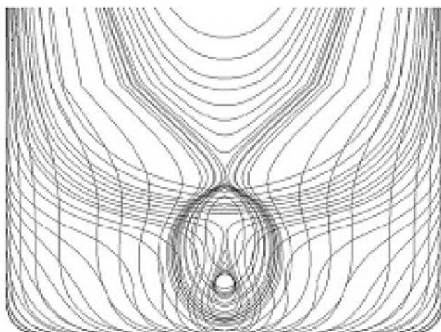
Figure 14 Body plan of the chemical tanker
