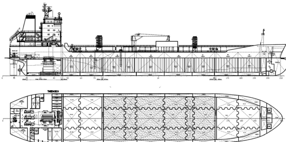
Figure 13 A 40 000 DWT chemical tanker designed by SSN
