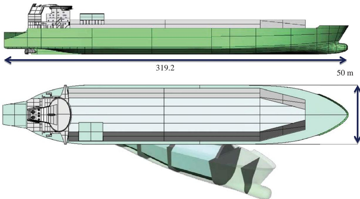
(SWBTs) arranged in the double-hull tanks, forward and aft. In the STX design, in the unloaded condition, the ship will be able to sail with a minimum volume of sea water or even without it. The use of these SWBTs is in a strong contrast with the ballast tanks onboard of a conventional LNG carrier, where the vessel is either full of LNG with empty SWBTs ("loaded") or empty of LNG with full SWBTs ("unloaded").
