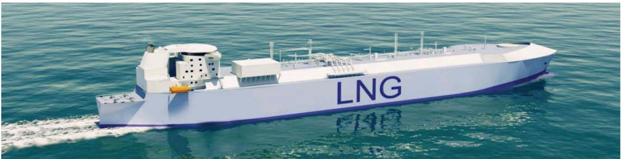
Figure 1 A 220 000 m<sup>3</sup> LNG carrier designed by *STX-France*
