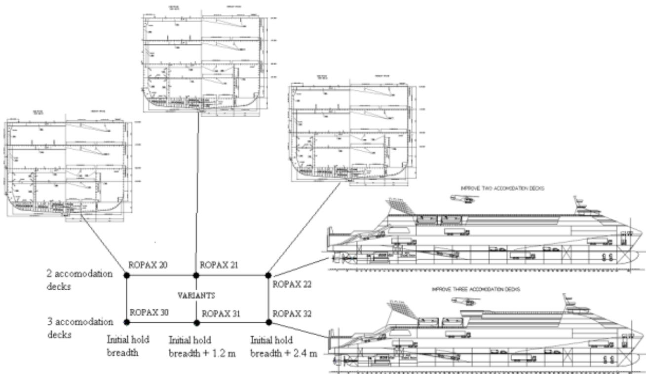
FEM models, see [21], in the generation of design alternatives on the Pareto frontier. In Ro-Pax case, they were further validated using the *IMPROVE* developed adequacy and quality measures (fatigue, robustness, LCC and production cost).
