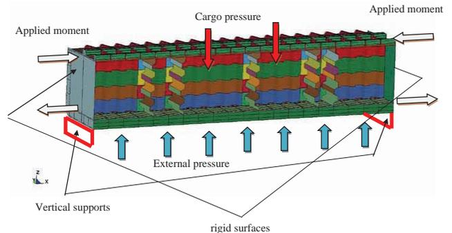
Figure 16 A 3D FE model of the chemical tanker
