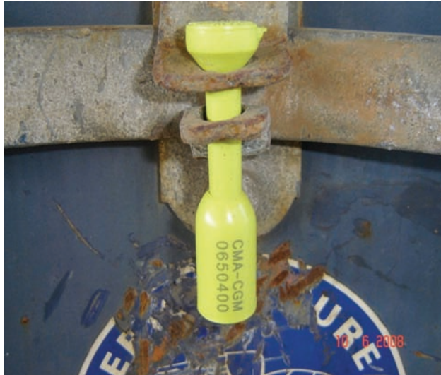
Picture 2: Ship's seal placed on the bottom of the containers' doors, blocking both sides of the door
