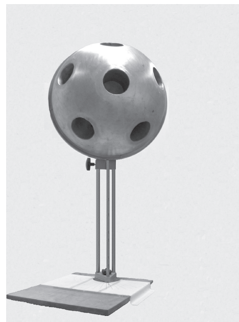
Fig. 3. Spherical experimental model (MODEL II) with six waveguides ( \alpha_1=0^\circ, \beta_{11}=0^\circ, \alpha_2=56^\circ, \beta_{21}=36^\circ, \beta_{22}=108^\circ, \beta_{23}=180^\circ, \beta_{24}=252^\circ, \beta_{25}=324^\circ ).
