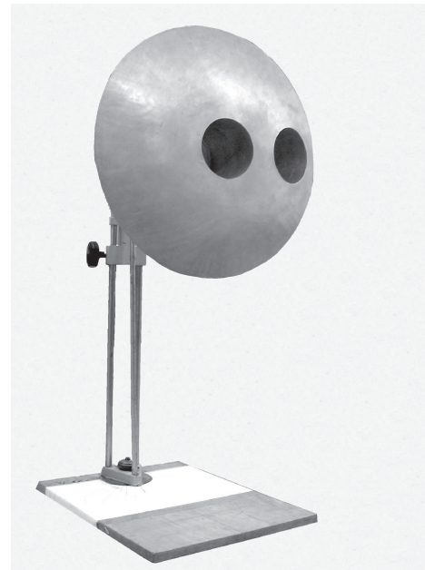
Fig. 2. Spherical experimental model (MODEL I) with two waveguides ( \alpha_1=0^\circ, \beta_{11}=0^\circ, \alpha_2=18^\circ, \beta_{21}=90^\circ ).
