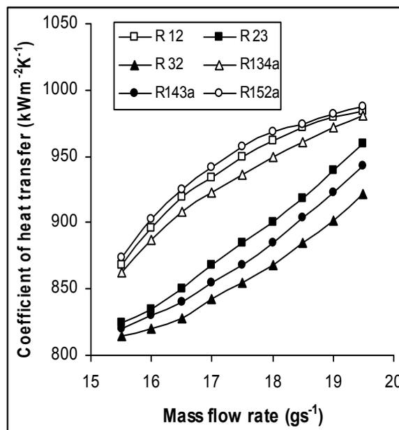
Figure 7. Effect of mass flow rate of refrigerants on overall coefficient of heat transfer of condenser
