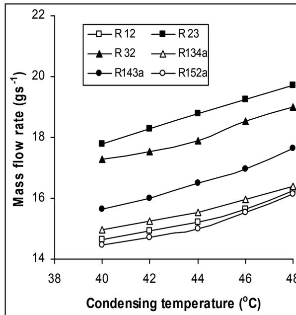
Figure 4. Effect of condensing temperature on the mass flow rate of refrigerants
