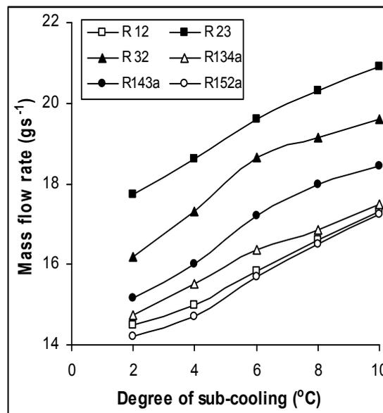
Figure 3. Effect of degree of sub-cooling on the mass flow rate of refrigerants
