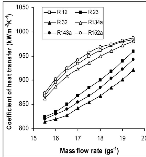
Figure 7. Effect of mass flow rate of refrigerants on overall coefficient of heat transfer of condenser
