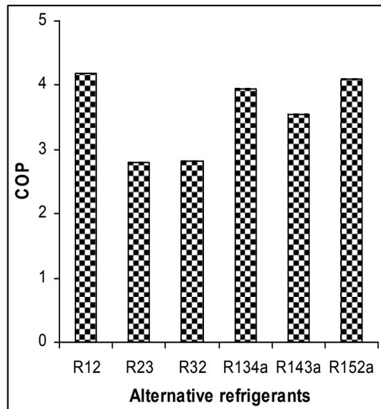
Figure 6. Coefficient of performance (COP) of alternative refrigerants
