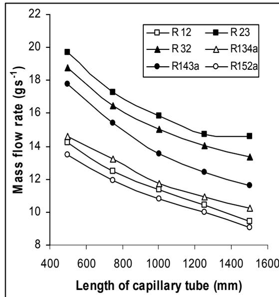
Figure 5. Effect of capillary tube length on the mass flow rate of refrigerants
