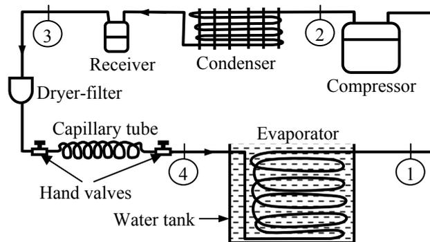
Figure 2. Experimental apparatus of vapour compression refrigeration system
