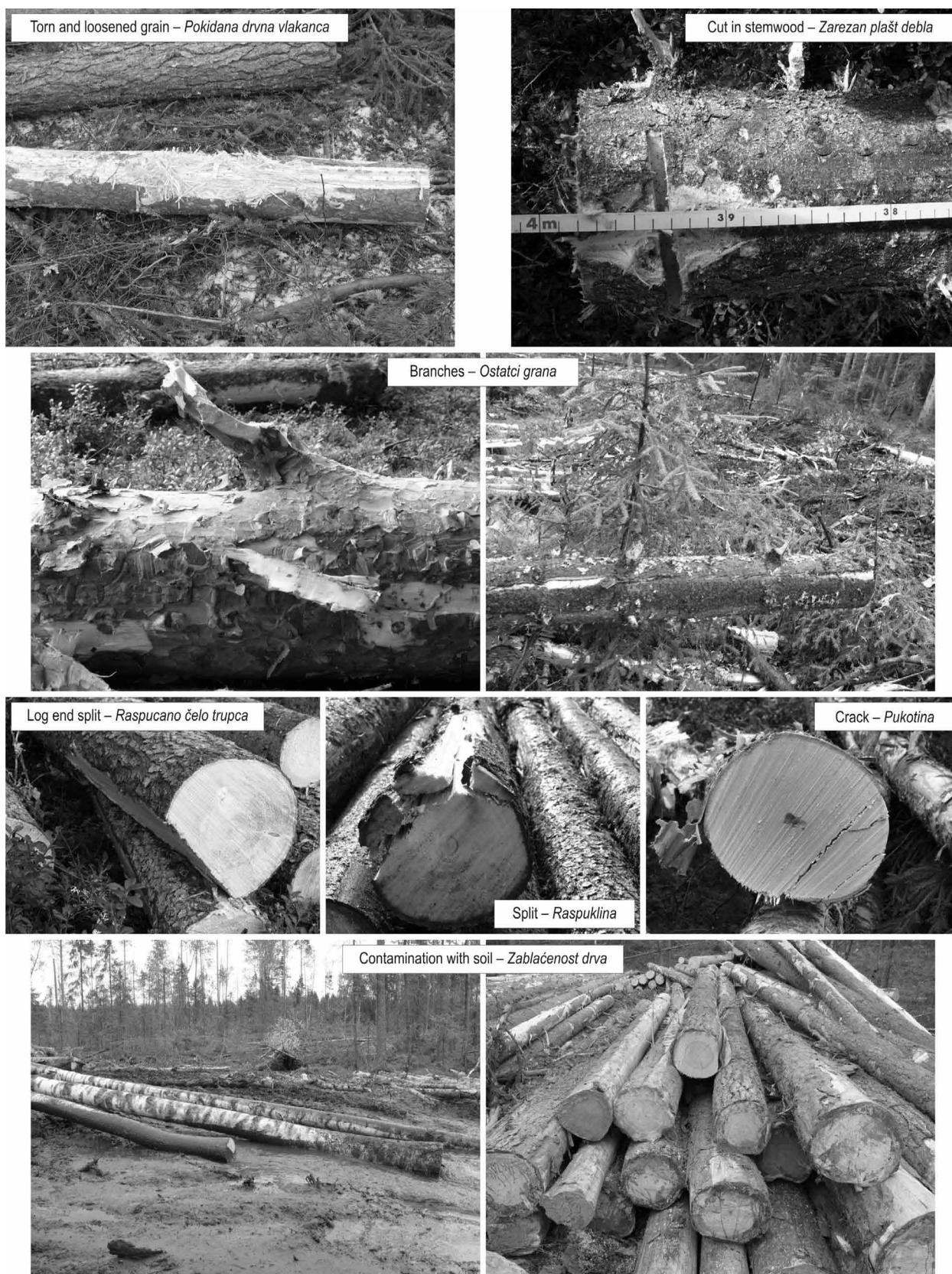
**Fig. 6** Typical IRW damages regulated by relevant national standards and log quality specifications
