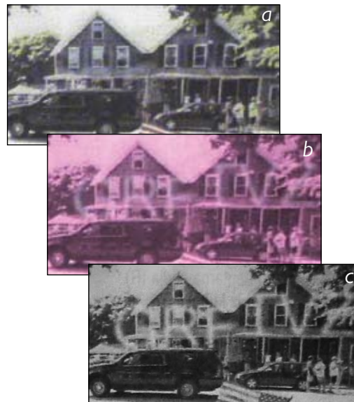
Figure 4. vs (a) and NIR exhibition (b, c) of the dual image design printed in the newspaper “Vjesnik” on August 21, 2010
