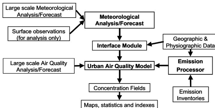
Figure 1. Air Quality Modelling system general architecture.
