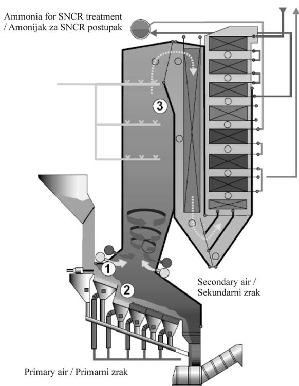
Figure 1. Von Roll waste combustion system [5]
