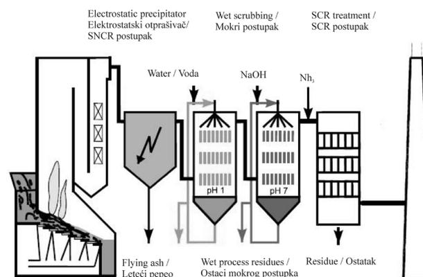
**Figure 3.** Variant 2 of the flue gas cleaning system
