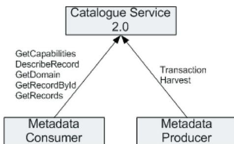
Fig. 4. CSW conceptual architecture.
