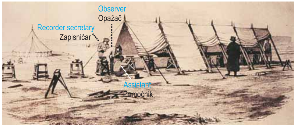
Fig. 13. Measuring the baseline using an apparatus which functioned on the principle of bi-metal temperature compensation, in 1828 (URL 30)
