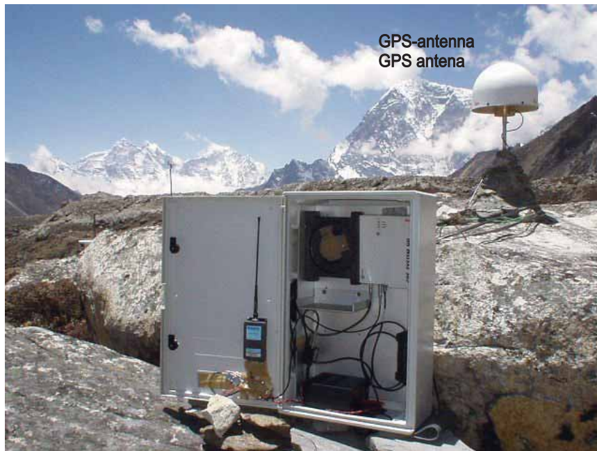
90 Fig. 34. Permanent GPS station located on the flank of the huge Khumbu glacier at the foot of Mt. Everest, which receives signals sent by GPS satellite, via a GPS hemispherical antenna (Photo: EV-K2-CNR Poretti/Leica Geosystems)
