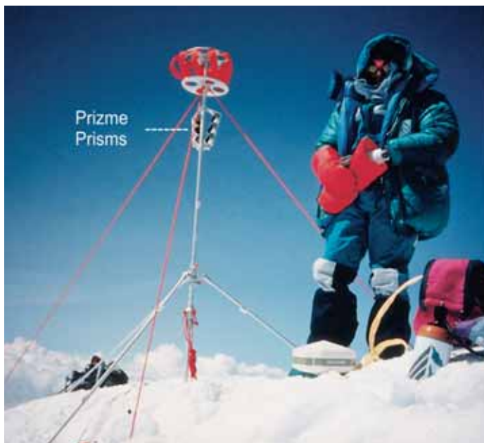
Fig. 27. Prism tripod for measuring distance using an electro-optical distance meter and the antenna of the GPS transmitter Leica System 200, on the summit of Mt. Everest (Photo: EV-K2-CNR Poretti/Leica Geosystems)
